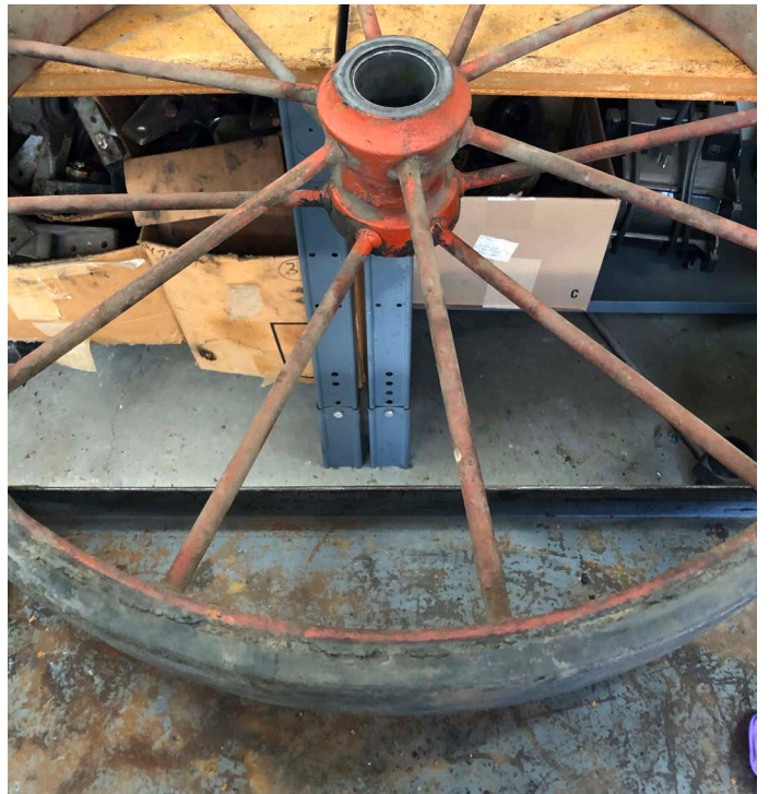
Original wood parts disassembled and the metal wheels with solid rubber tires
